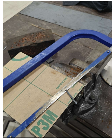
(b) Cutting of Acrylic Sheets
