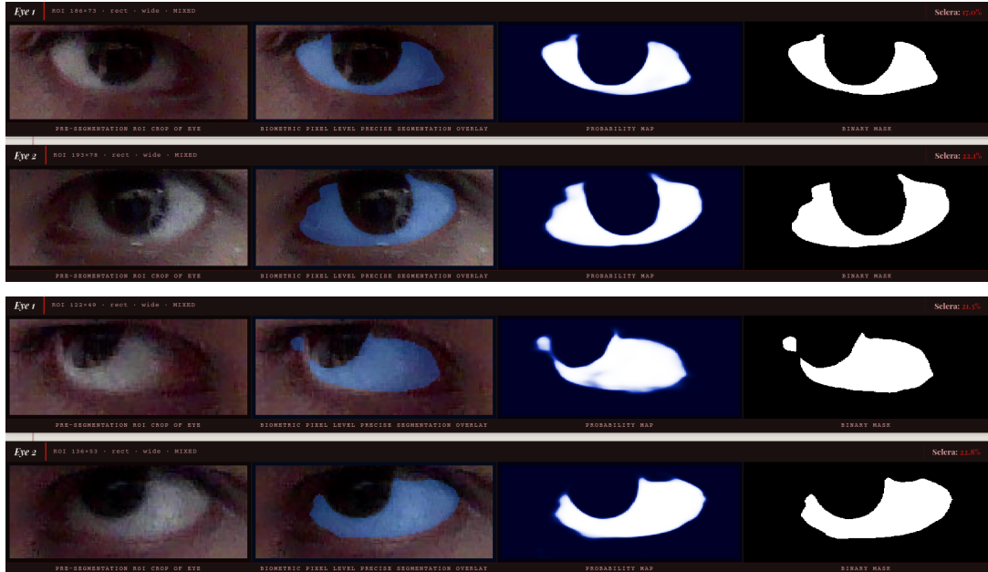
Figure 24: Mixed model — qualitative segmentation overlays. Two eye samples from the mixed regime (wide-rectangular ROIs, 122 \times 49 and 186 \times 73 ). Each row: pre-segmentation ROI crop | biometric pixel-level overlay (blue sclera) | probability map | binary mask. Sclera fractions: 21.3% (Eye 1) and 17.0% (Eye 2). Wide-rectangle crops represent the challenging unconstrained real-world acquisition conditions (MASD/SBVPI); the mixed model correctly segments the exposed sclera region despite significant pose and illumination variability.
