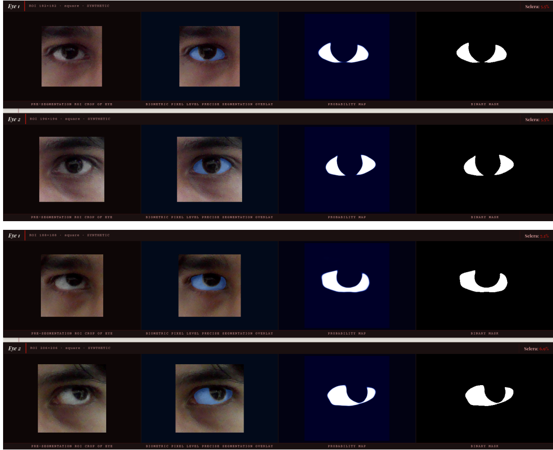
Figure 23: Synthetic-only model — qualitative segmentation overlays. Two eye samples from the synthetic regime (square ROIs, 168 \times 168 and 182 \times 182 ). Each row: pre-segmentation ROI crop | biometric pixel-level overlay (blue sclera) | probability map | binary mask. Sclera fractions: 7.2% (Eye 1) and 3.5% (Eye 2). Note the sharp, confident boundary delineation and minimal false-positive regions.
